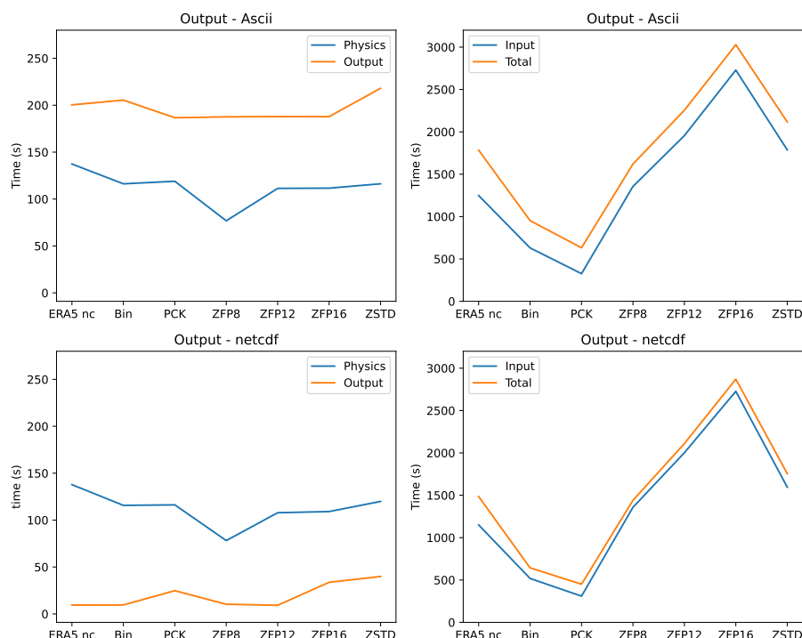
Figure 4. MPTRAC runtime comparison using the ERA5 netcdf files, the bin files and the compressed PCK, ZSTD and ZFP files for the 10-day forward trajectory calculations with MPTRAC. Top panels for trajectory output stored as ascii and bottom panels for trajectory output stored as netcdf file.
