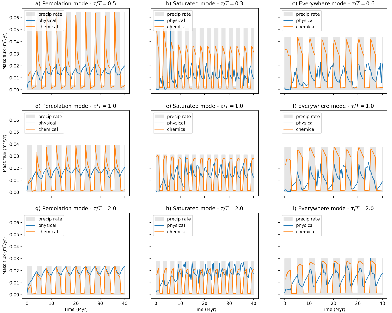
Figure 21. Predicted variations in chemical and physical fluxes as a function of time for model runs experiments with periodic precipitation rate. Each column corresponds to a different mode ( C ) and each row to a different ratio of the laterisation time scale ( \tau ) by the period ( T ). Note that, as in model experiments shown in Figure 14 and 15, in each mode, the period of forcing was selected to be equal to the laterisation time scale that lead to the formation of a thin duricrust, i.e., T = 4, 4 and 7 Myr, respectively. Grey shaded areas indicate periods of enhanced precipitation rate.
