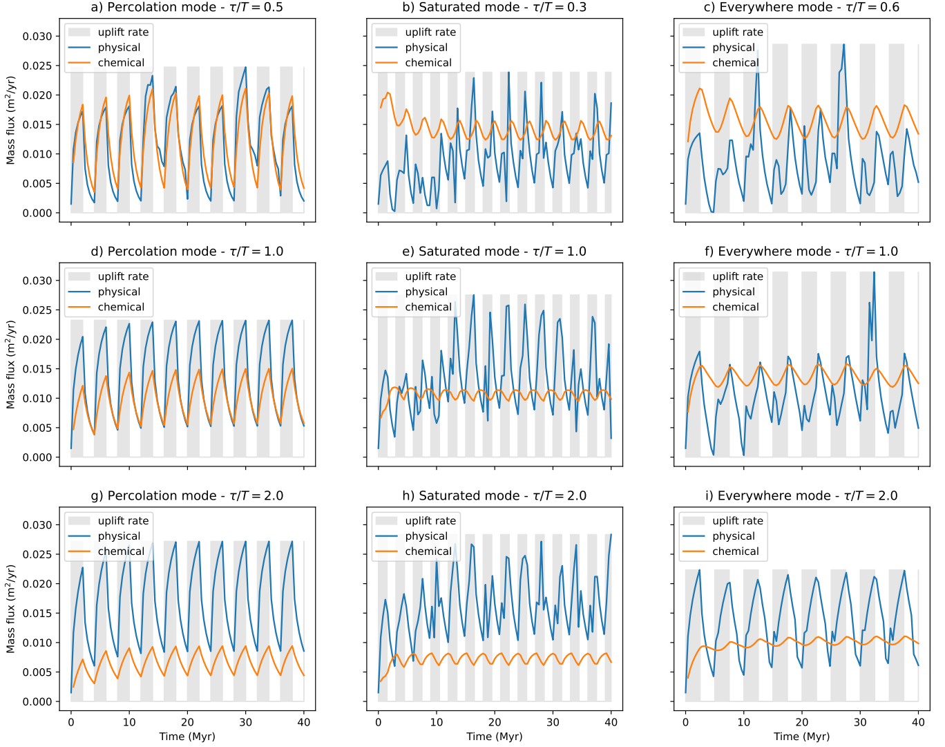
Figure 20. Predicted variations in chemical and physical fluxes as a function of time for model runs experiments with periodic uplift rate. Each column corresponds to a different mode ( C ) and each row to a different ratio of the laterisation time scale ( \tau ) by the period ( T ). Note that, as in model experiments shown in Figure 11 and 13, in each mode, the period of forcing was selected to be equal to the laterisation time scale that lead to the formation of a thin duricrust, i.e., T = 4, 4 and 7 Myr, respectively. Grey shaded areas indicate periods of enhanced uplift rate.
