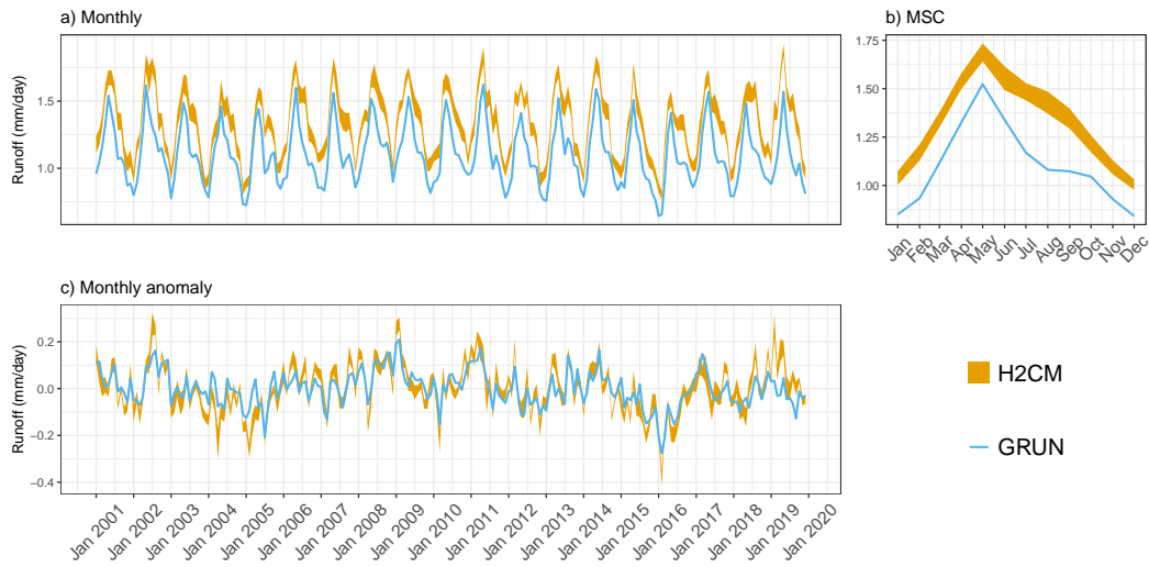
Figure C8. Predicted versus target mean runoff over the testing set (spatial domain) across 10 CV folds: a) monthly, b) mean seasonal cycle over the entire period of data constraint and c) monthly anomaly.
