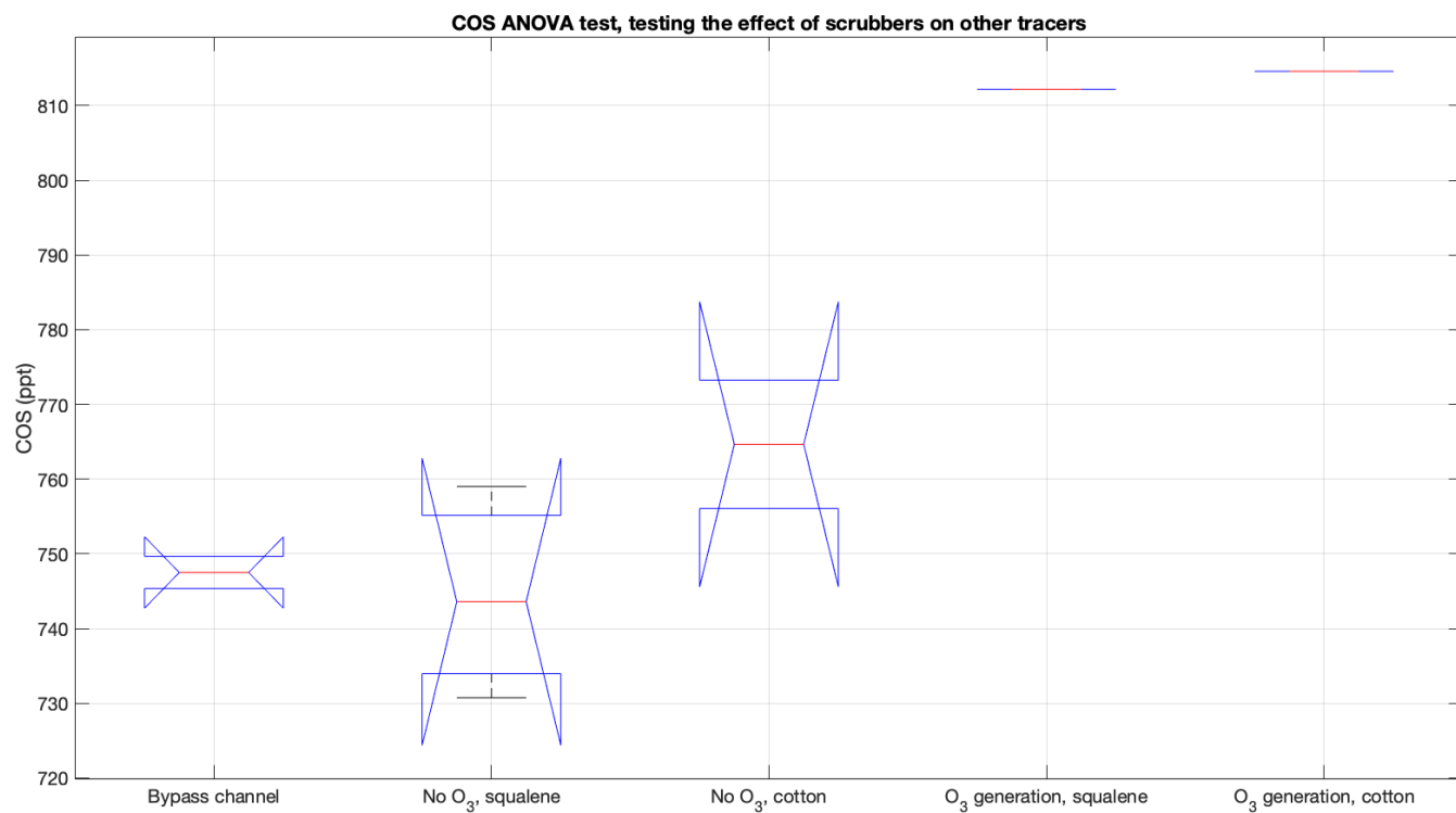
Figure 4: effects of squalene and cotton O 3 scrubbers on a compressed tropospheric air mixture containing COS.
