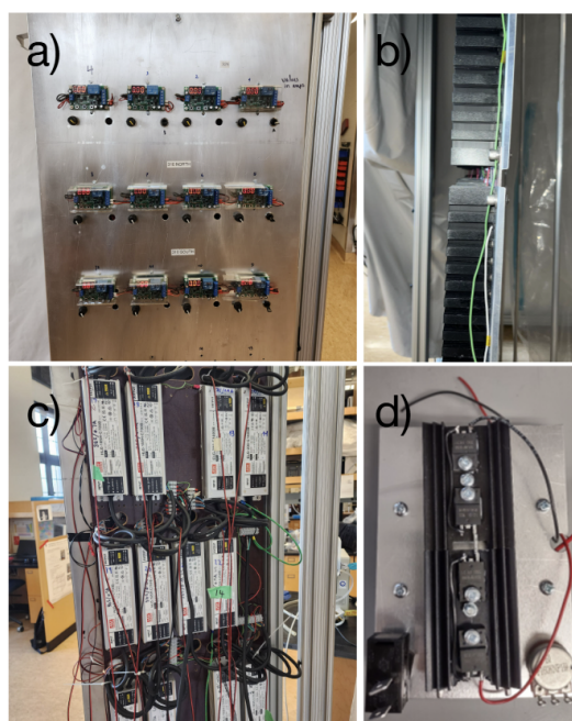
Figure 2. The electrical control panel for the LEDs are shown in the images. (a) A user-accessible control panel reads out the current driven through each LED. Each current display module is linked to a panel of 3 bars consisting of 12 LEDs each. The black switch turns the LEDs on and off, while the knobs adjusts the current. The LEDs are made of three components: (b) The heatsinks are connected to the LED bar via an aluminum mounting frame (side view). (c) Power supply units are mounted at the rear of the panel shown in (a). (d) Heatsinks are shown with the wiring depicted in Figure S8 to connect to an LED bar.
