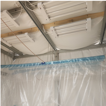
Figure S2. The photograph shows the pulley system that lifts and collapses the bag in the ATMOX chamber.
