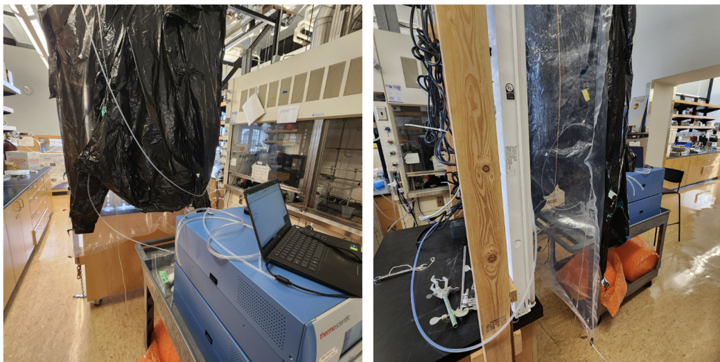
Figure S12. Actinometry measurements were performed on a 0.45 m 3 PFA bag using fluorescent lights. Photo on the left depicts the 42I and 49I gas analyzers, while the photo on the right depicts the side view of the fluorescent lights and pillow bag.
