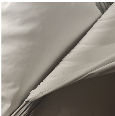
Figure S3. The image shows the blackout curtains used in the ATMOX chamber. The loops sewn onto the blackout blinds wrap around the aluminum rods mounted at the top of the chamber.
