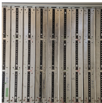
Figure S5. The photograph shows the LED bars (1 bar contains 12 LEDs) mounted on custom built aluminum panels. Then, three bars were wired in series on each panel, illustrating the electrical grouping used in ATMOX.
