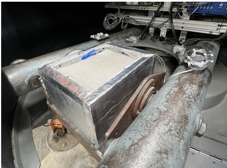
Figure 1. Insulated sample place on 1-m radius centrifuge. Aluminium container is surrounded by insulation (silver panels on outside of soil container), while wiring for resistance temperature detectors can be seen emerging from the soil near the back left.
