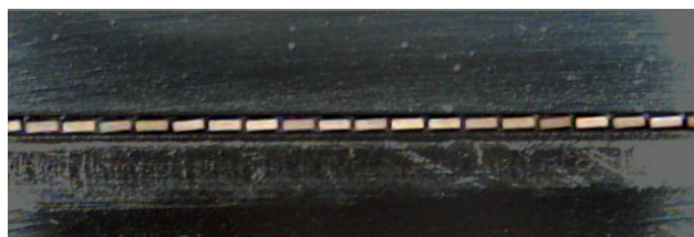
Figure 2. Image of a section of aligned fibers within the aluminum ferrule from Fig. 1. The fiber core dimension is \sim 300 \mu\text{m} \times 100 \mu\text{m} .
