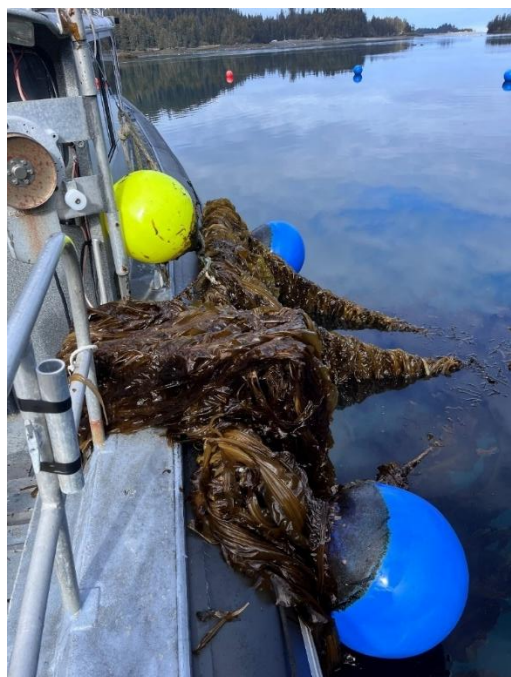
Figure A2. The biofouled moorings retrieved from Jakolof Bay in spring 2024. Wild-set Alaria marginata completely encompassed the mooring frames and sensors.
