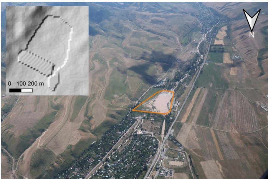
145 Figure 5: Photograph of the dam and retention basin (outlined in orange) in the village of Kashka Suu. Box top left: Hillshade of the artificially modified DEM for the RAMMS simulation of the DRM measure of the retention basin. Photograph: V. Zaginaev, July 2024.
