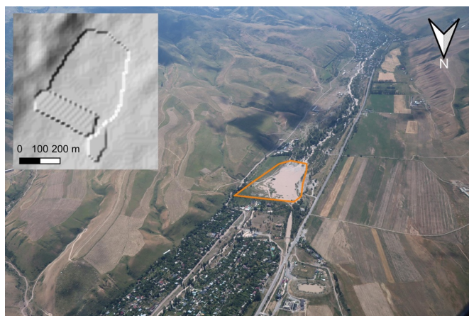
Figure 5: Photograph of the dam and retention basin (outlined in orange) in the village of Kashka Suu. Box top left: Hillshade of the artificially modified DEM for the RAMMS simulation of the DRM measure of the retention basin. Photograph: V. Zaginaev, July 2024.
