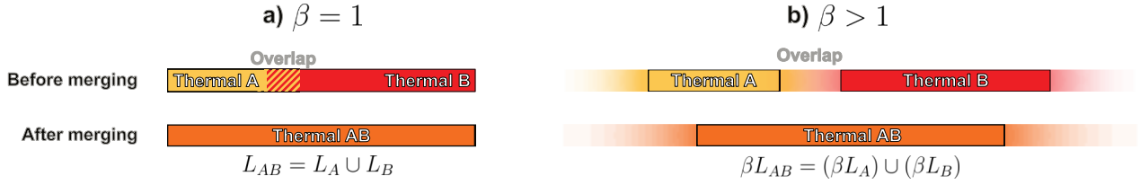
Figure A1. Illustration of the merging process assuming two objects merge (a) if and only if they overlap or (b) if their basins of attraction overlap – the basin of attraction (or effective length) of object A has a length \beta L_A , where L_A is the actual length of object A and \beta is the effective factor (shown in shading, defined in Appendix A and further interpreted in section 6.2). The rules for object merging are as follows. When \beta = 1 , the length of the merged ( L_{AB} ) object will be the union of the two incipient objects' lengths ( L_A \cup L_B ). When \beta > 1 , the length of the merged object's basin of attraction ( \beta L_{AB} ) will be the union of the two incipient objects' basins of attraction ( \beta L_A \cup \beta L_B ).
