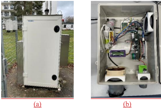
Figure 1. Photographs of the AEMS and AELCM units (AELCM009 and AELCM010), which are mounted on the fence next to the AEMS: (a) the stationary air and climate measurement station of the Chair for Regional Climate Change and Health, Faculty of Medicine, University of Augsburg; and (b) the housing and interior view of the engineered AELCM units.
