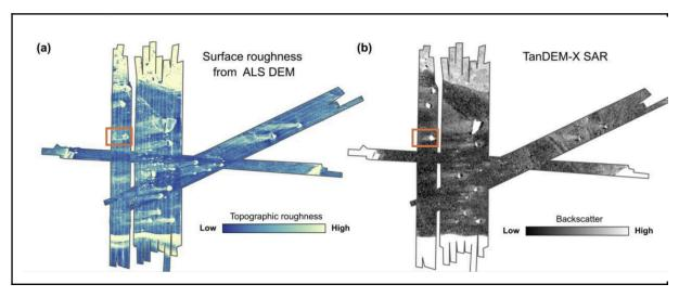
Figure from the reviewer's supplement highlighting high SAR backscatter on the lee of an iceberg, which is unrelated to topographic roughness of the surface (red rectangles).
