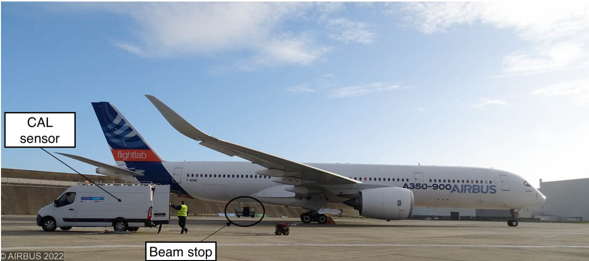
Figure 2. Picture of the test setup at the Airbus SAS Bikini outdoor test facility with an Airbus A350-900 Flight Lab test aircraft. The arrows indicate the location of the CAL sensor and a beam stop for laser safety.
