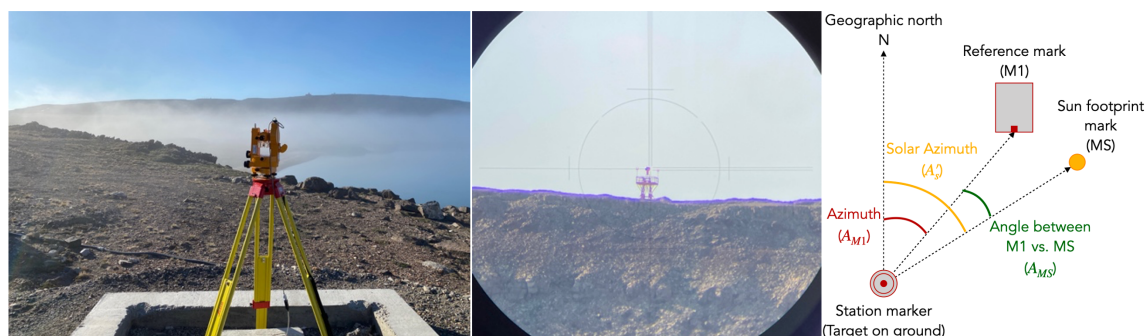
Figure 3: Sun observations for azimuth determination. Left: The fluxgate theodolite mounted above the Pillar A foundation at PIF, aligned toward a distant reference mark located several kilometres away. Centre: View of the reference mark through the theodolite's monocular. Right: Illustration (by Marie V. Eldor) showing the key angles involved in a sun observation. A_{M1} is the essential azimuth angle for accurate declination measurements.
