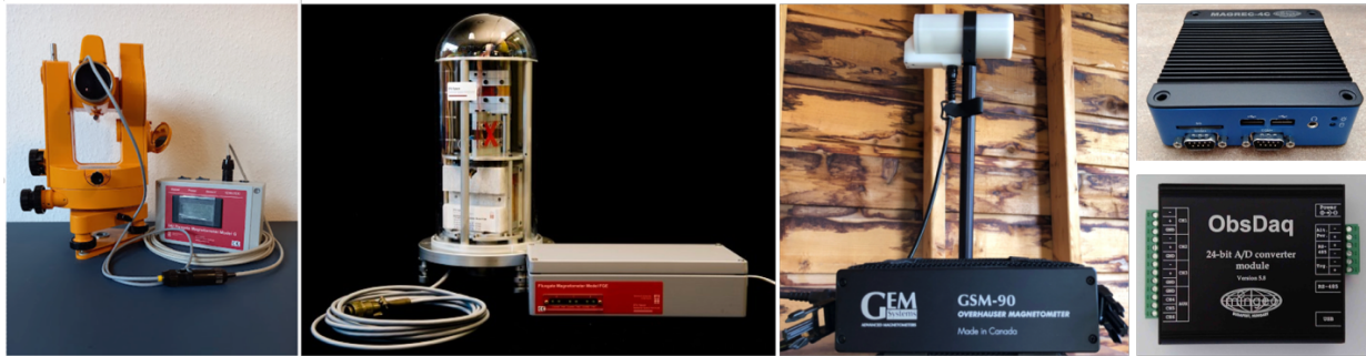
Figure 4: DI instrument: Fluxgate theodolite (converted Zeiss THEO 020) with DI Magnetometer Model G (to the left, picture from DTU Space), Variometer: 3-axis Fluxgate Magnetometer Model FGM-FGE (left middle, picture from DTU Space), Scalar instrument: GEM Systems Overhauser GSM-90 Scalar Magnetometer (right middle, the picture is from GEM systems), Datalogger: MinGeo Magrec-4C with ObsDaq 24-bit fast A/D converter (to the right, the pictures are from MinGeo).
