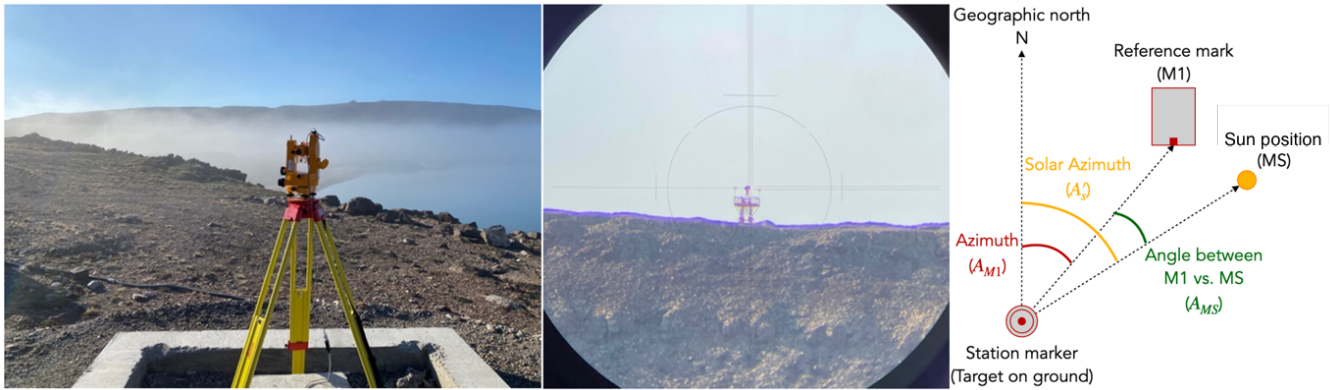
Figure 3: Sun observations for azimuth determination. Left: The fluxgate theodolite mounted above the Pillar A foundation at PIF, aligned toward a distant reference mark located several kilometres away. Centre: View of the reference mark (M1) through the theodolite's monocular. Right: Illustration (by Marie V. Eldor) showing the key angles involved in a sun observation. AM1 is the essential azimuth angle for accurate declination measurements.
