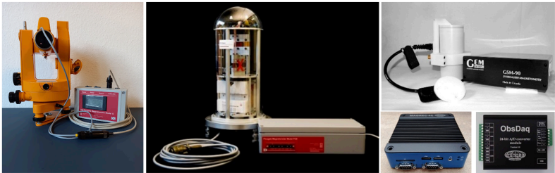
Figure 4: DI instrument: Fluxgate theodolite (converted Zeiss THEO 020) with DI Magnetometer Model G (to the left, picture from DTU Space), Variometer: 3-axis Fluxgate Magnetometer Model FGM-FGE (middle, picture from DTU Space), Scalar instrument: GEM Systems Overhauser GSM-90 Scalar Magnetometer (to the upper right, the picture is from GEM systems) , Datalogger: MinGeo Magrec-4C with ObsDaq 24-bit fast A/D converter (the pictures are from MinGeo).
