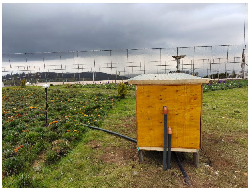
Figure 2. Magnetometer Setup: The magnetometer is housed in a protective structure designed to withstand environmental challenges, including potential flooding, and to maintain temperature stability. Data is logged continuously and transferred to the respective institutes for analysis and storage.
