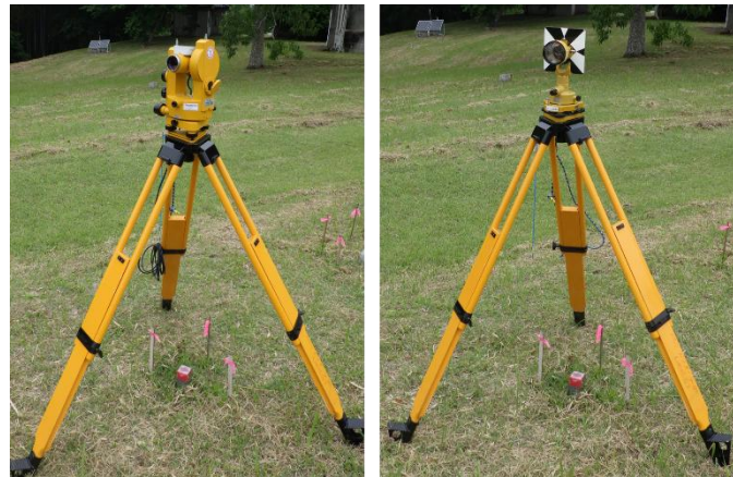
Figure 5: A set of instruments for the horizontal angle observation.
