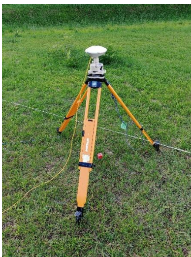
Figure 3: A photo the GNSS equipment mounted on a tripod.
