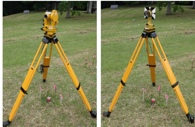
Figure 5: A set of instruments for the horizontal angle observation. THEO-010B theodolite on the left and a survey prism on the right
