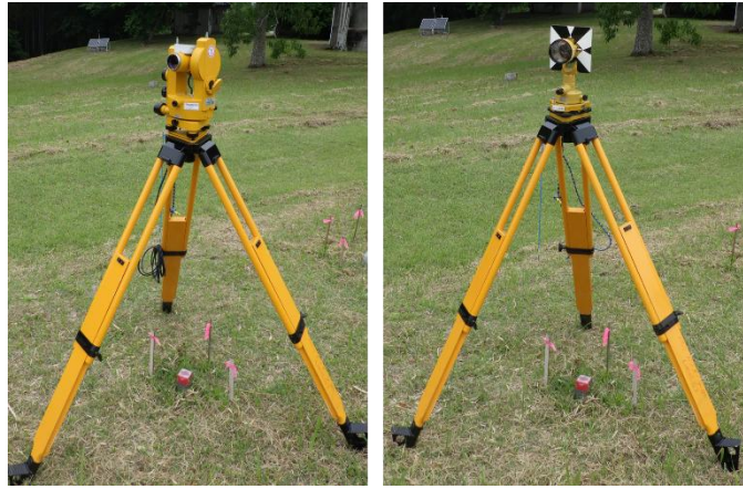
Figure 5: A set of instruments for the horizontal angle observation.
