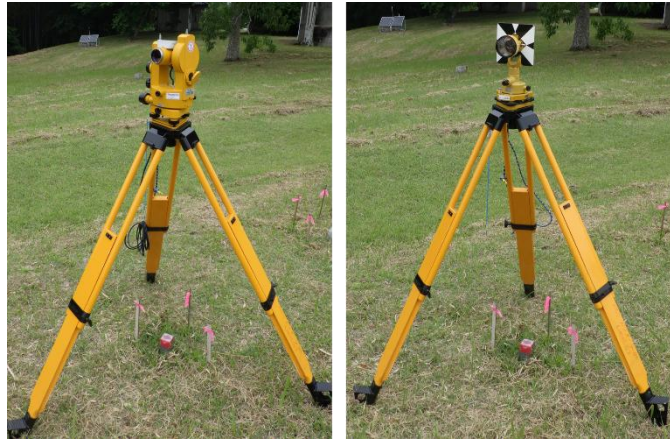
Figure 5: A set of instruments for the horizontal angle observation. THEO-010B theodolite on the left and a survey prism on the right
