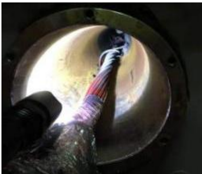
(a) Burnt shipboard transmission cable (b) Power booster overheating Figure 2: The risks of thermal overload in MCSEM system.
