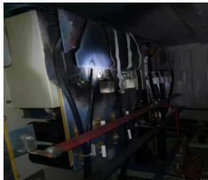
(a) Burnt shipboard transmission cable (b) Power booster overheating Figure 2: The risks of thermal overload in MCSEM system.
