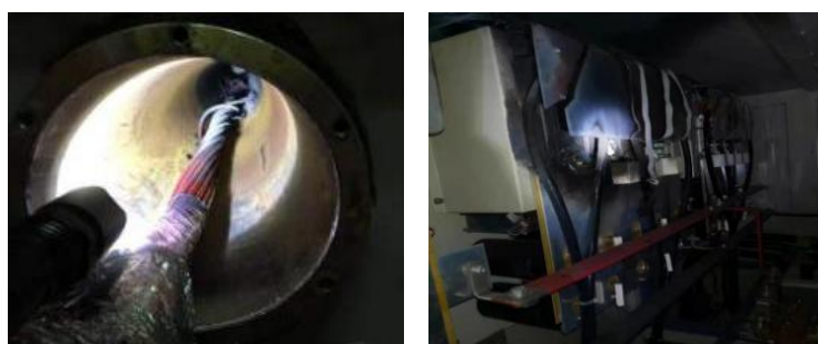
(a) Burnt shipboard transmission cable (b) Power booster overheating Figure 2: The risks of thermal overload in MCSEM system.
