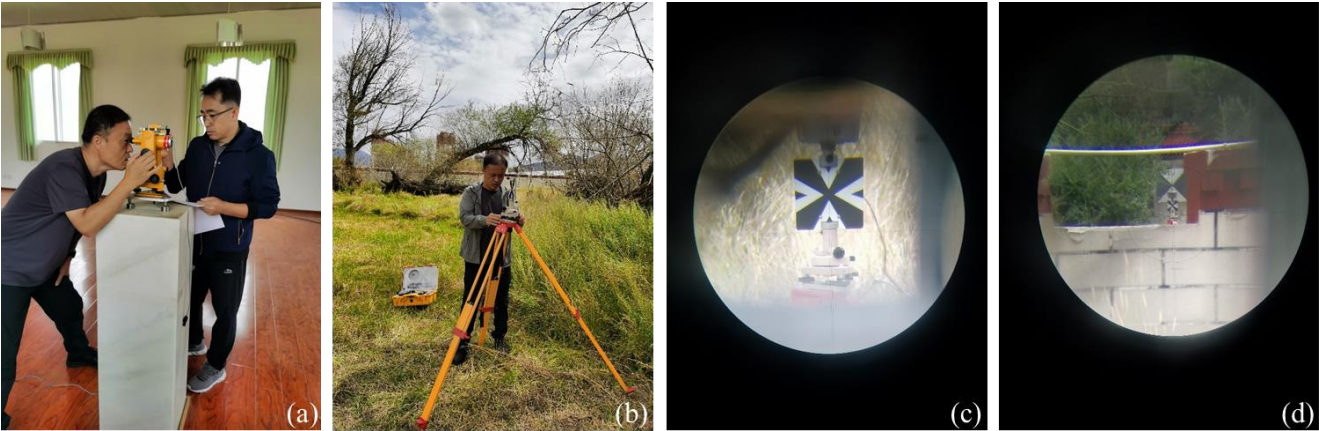
Figure B1: Theodolite alignment to the GNSS targets and the azimuth mark.
