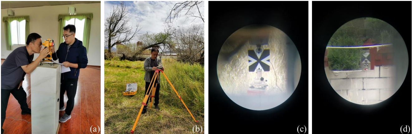
Figure 4: Theodolite alignment to the GNSS targets and the azimuth marker.
