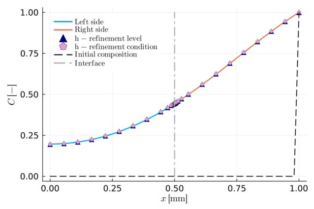
Example B1 solved for the case of the two h-refinement approaches (see main text for more details). In the "h-refinement level" solution we performed the refinement by choosing a fixed number of refinement levels. In the "h-refinement condition" we performed the refinement until the length ratio of the largest to the smaller element is the same as the one that was chosen by the user. The solid lines indicate our original refinement approach (m-refinement).
