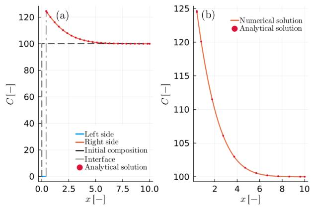
Same calculation as for example B5 (Fig. 7 in the new version of the manuscript). This example was calculated with the h-refinement approach using initially 50 nodes and 3 refinement levels.
