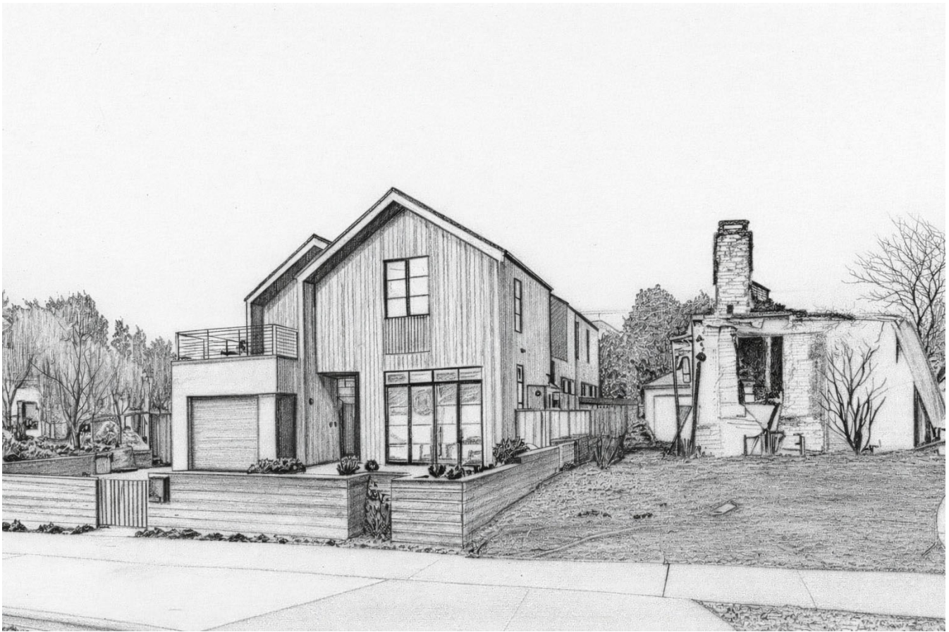
70 Figure 1. The sketch shows a wildfire-surviving house in Pacific Palisades, Los Angeles, constructed according to wildfire-resistant design principles. It is illustrating the concept of a non-combustible or fire-resistant exterior façade, helping to reduce ignition from radiant heat and wind-driven embers. Multi-pane windows are used to increase resistance to heat exposure and minimize breakage. The design includes adapted roof overhangs, sealed eaves, and ember-resistant detailing that limit pathways for embers to enter the structure. Gutters are designed to reduce debris accumulation, further lowering fire risk. Further details for reducing vulnerability are described in Papathoma-Köhle et al. (2022, 2025). Together, these architectural strategies contributed to the building’s remarkable performance during the 2025 wildfire events. Figure conceptualized from a Google Street View scene (02/2025). 75
