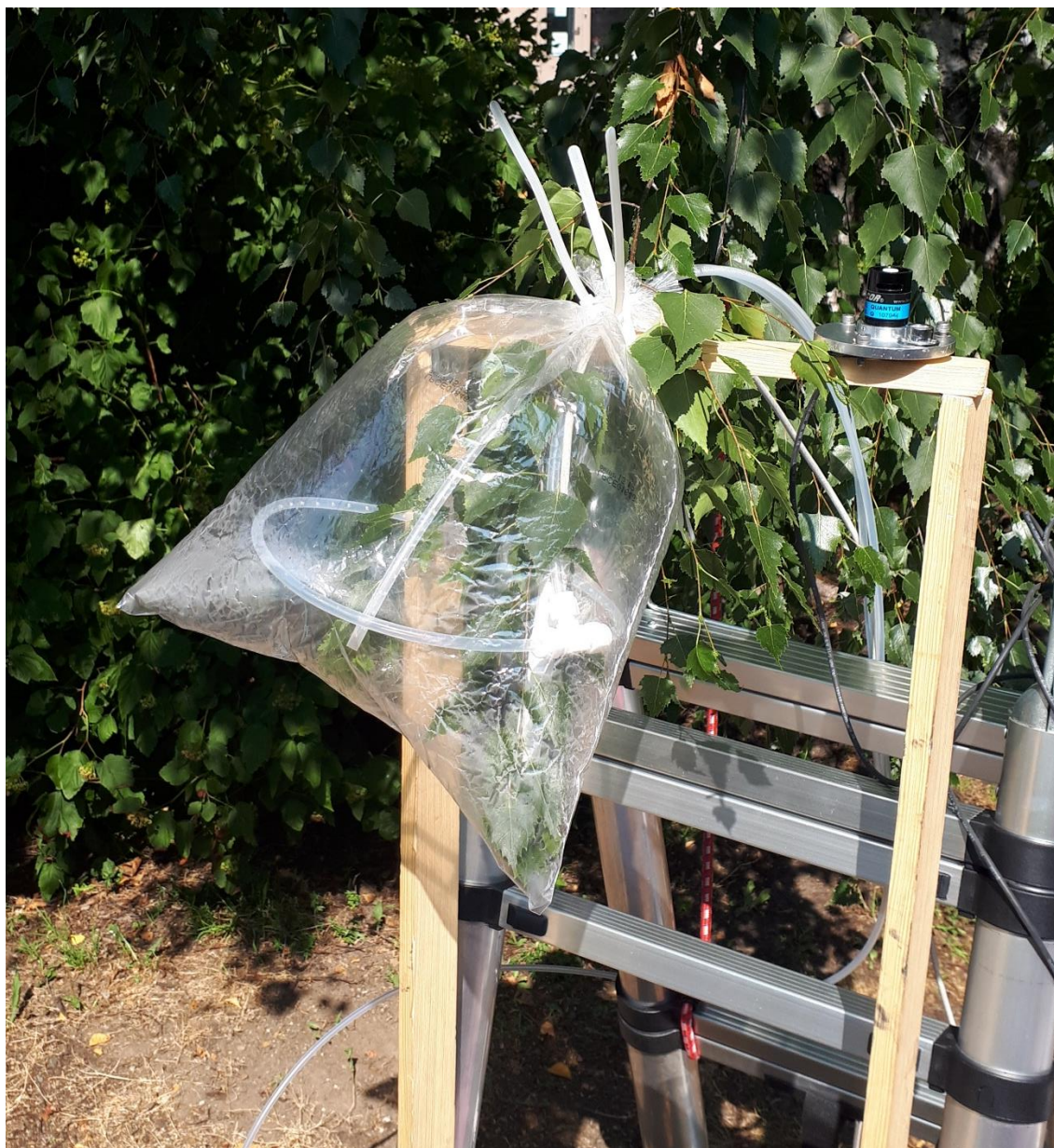
Figure S2. The measurement system: FEP tubing, PET bag, T and RH sensor (inside the bag), and PAR sensor (on top of the wooden support) attached to a Betula pendula branch in Helsinki in July 2022.
