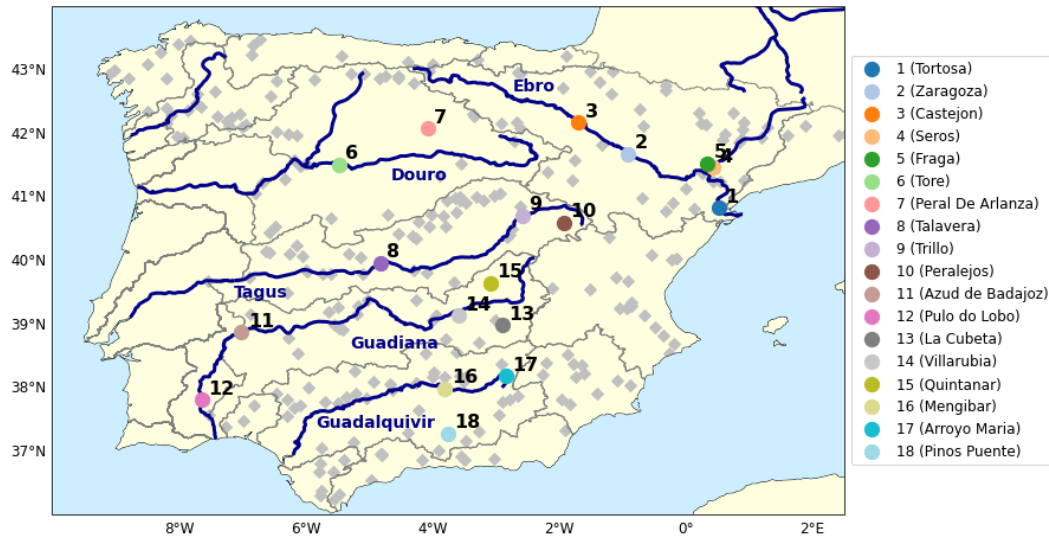
Figure 2. Stations used for river discharge evaluation and major rivers of the Iberian Peninsula, with river basin district borders from the WISE WFD Reference Spatial Datasets reported under Water Framework Directive. Grey diamonds show river dams from FAO - Aquastat (2009).
