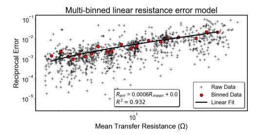
The multi-binned linear resistance error model defines a slope and intercept that is used to estimate errors for individual measurements. From the error model above, we can use a histogram of the relative error applied to see the distribution of likely errors for all measurements. The graph below indicates 97.2% of the data has a relative error of less than 2%.
