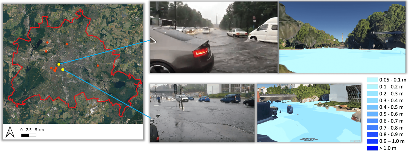
Figure 4. The red line indicates the administrative boundary of Berlin, while the red dots mark the 19 locations where photos or videos from the June 2017 flood were available and were compared to RIM2D simulation results. Two example comparisons are shown for Berlin Hofjägerallee (top) and Berlin Yorckstraße (bottom), illustrating how the dx = 5 m RIM2D simulation results align with observations from social media. The RIM2D outputs are visualized using Google Earth, with background imagery provided by Google Earth (Satellite imagery: © Google Earth 2025). Social media content used for validation is © X Corp. 2025 and reproduced under fair use for academic purposes.
