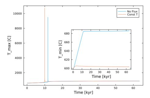
Maximum and minimum (inset) temperature for no-flux boundary condition (blue, used in our study) and constant temperature boundary condition (orange) in a 1D model. Temperature is saved at cell centers, so even for constant T boundaries, there is a little bit of increase in T\_min.
