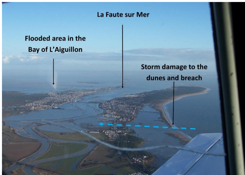
40 Figure 1 Aerial photograph (28 February 2010) illustrating how the erosion of Belle Henriette (right) created an additional pathway for floodwaters (blue arrow) into La Faute-sur-Mer, France during Storm Xynthia 2010 (Photo J-P Bichon, interpretation M. Garcin, BRGM; see also Pedreros et al., 2010, Gerard and Lang, 2019)
