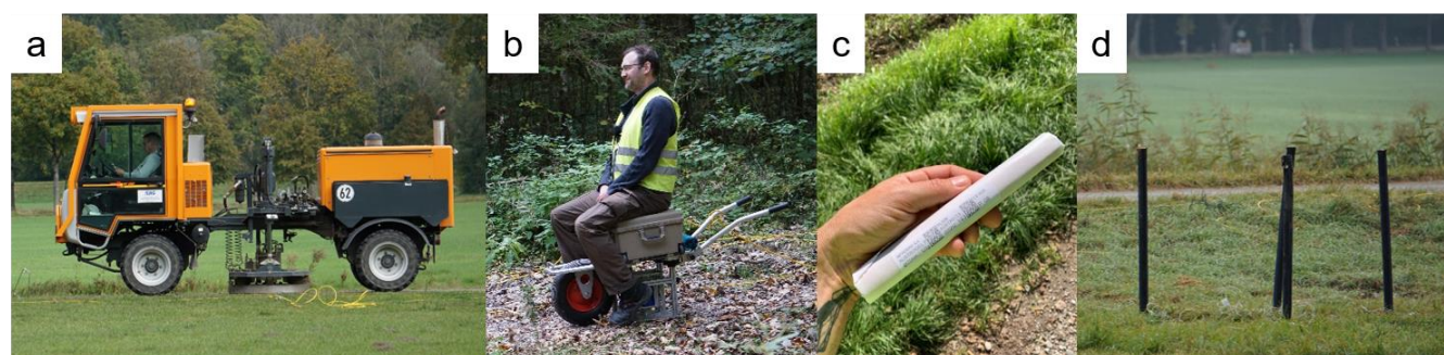
Figure 1: Seismic sources. Vibrators MHV4P (a), ELVIS-7 (b), explosives (c), and boreholes prepared for charging (d).
