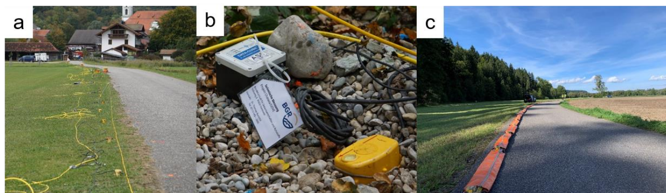
125 Figure 2: Seismic receivers. Regularly planted vertical geophones connected by cable (a), 3-component geophone and recording unit (b), and landstreamer with horizontal 1-component geophones (c).
