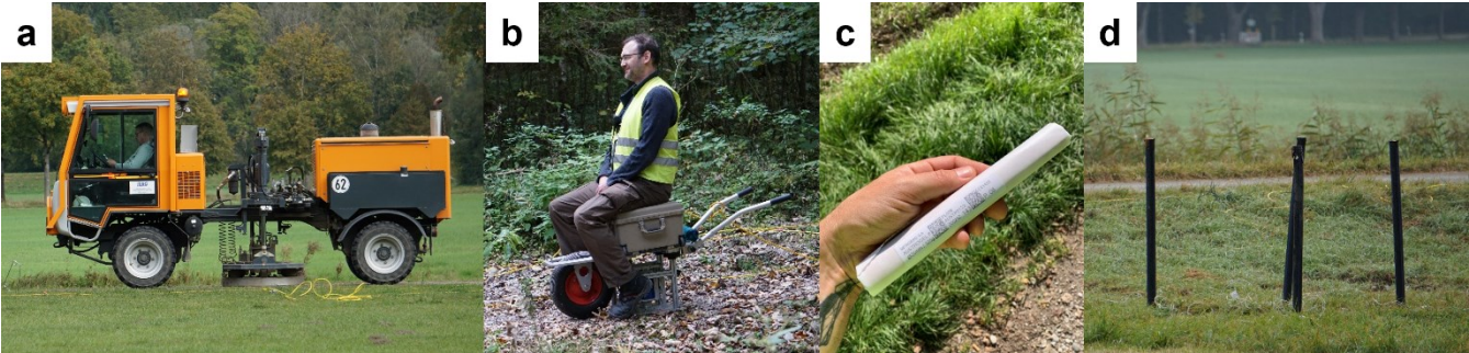
Figure 2: Seismic sources. (a) Vibrators MHV4P, (b) ELVIS-7, (c) explosive charge, and (d) boreholes prepared for charging.
