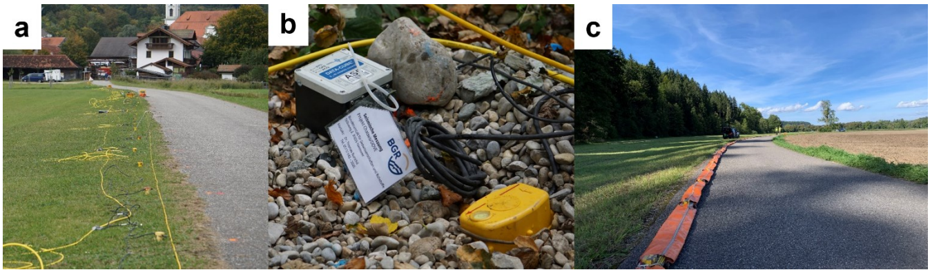
Figure 3: Seismic receivers. (a) Planted vertical geophones connected by cable, (b) 3-component geophone and DATA-CUBE 3 , and (c) landstreamer with horizontal geophones.
