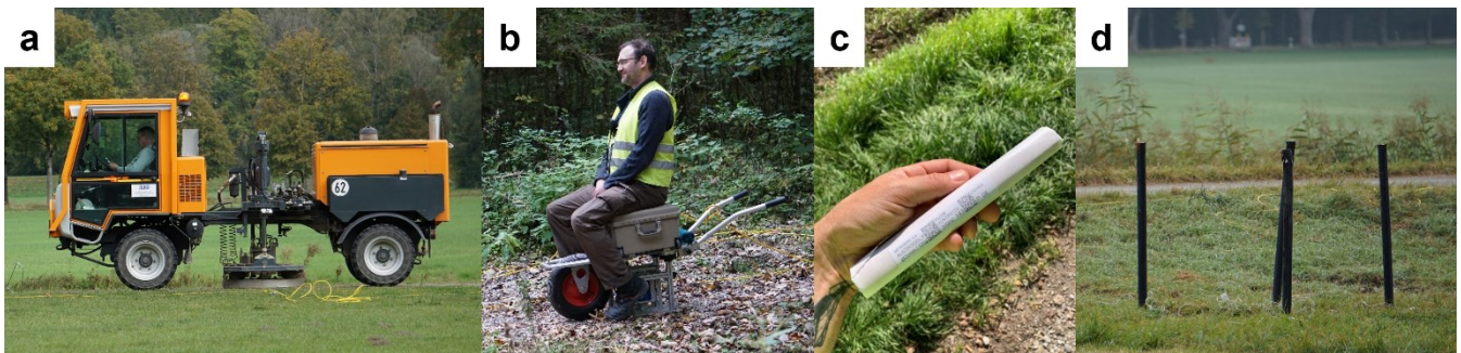
Figure 2: Seismic sources. (a) Vibrators MHV4P, (b) ELVIS-7, (c) explosive charge, and (d) boreholes prepared for charging.
