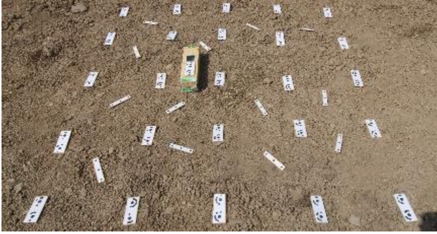
Figure 5: Control point scheme for camera calibration adjacent to the experimental field.
