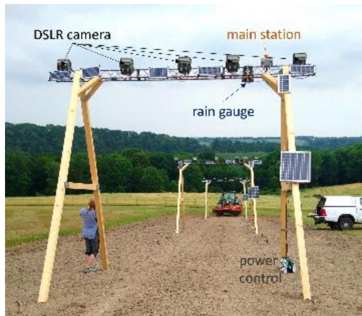
90 Figure 1: Construction of the soil surface monitoring system at the lower, middle, and upper slope positions observing the hillslope field with synchronized DSLR (digital single-lens reflex) cameras that were triggered by a rain gauge. The image shows the regular upslope and downslope tillage of the field.
