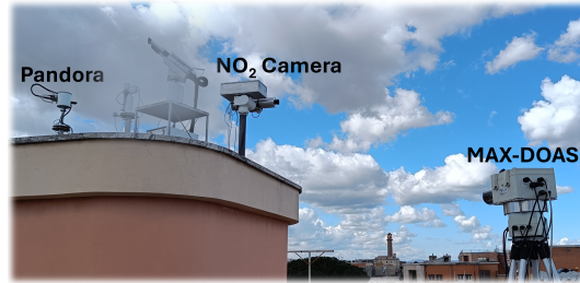
Figure 2. The NO 2 camera and the two reference instruments installed for the campaign at the BAQUNIN-APL supersite.
