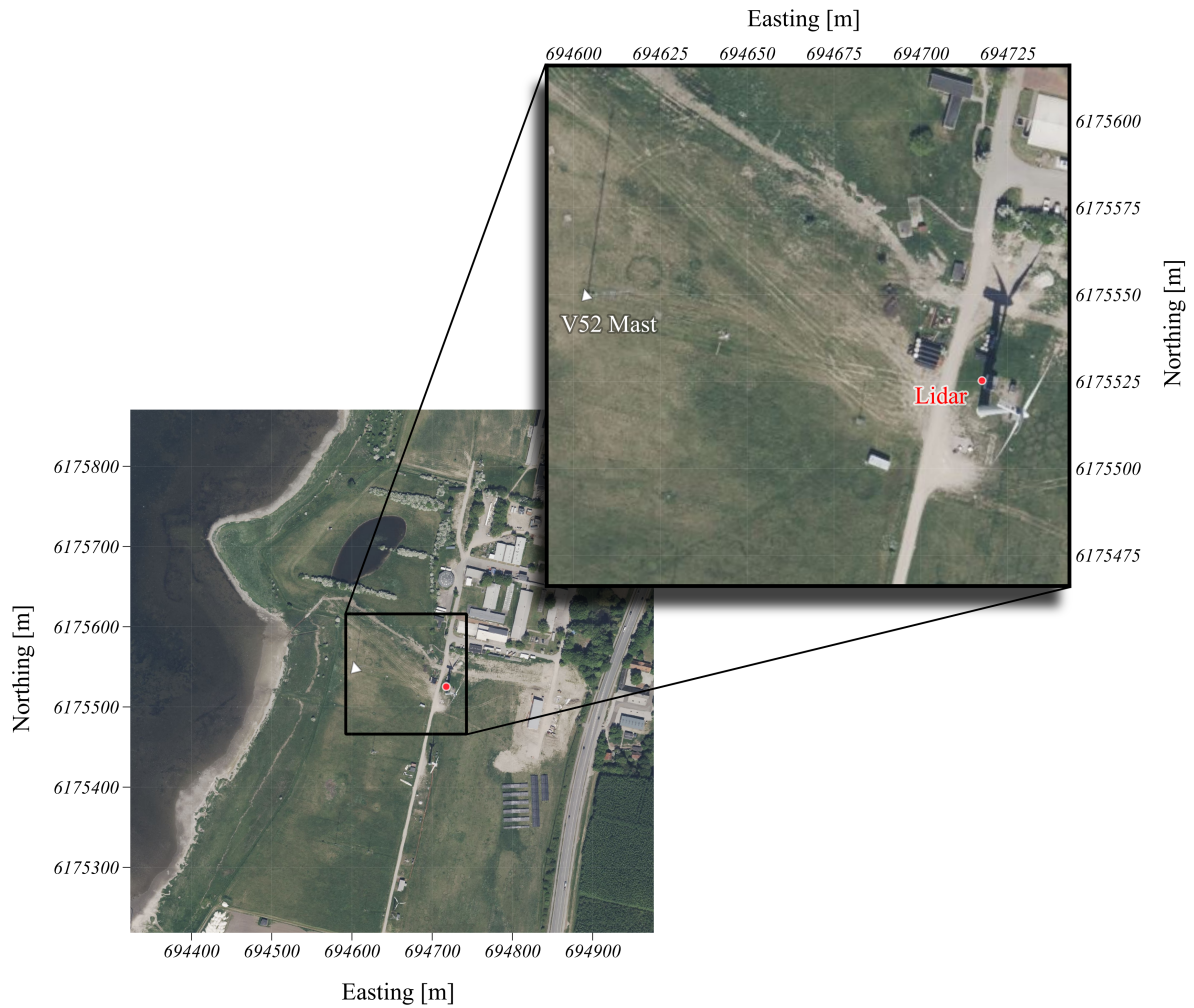
Figure 4. Satellite image of the experimental field at Risø campus (Denmark) provided by Bing Maps, copyright 2025 © Microsoft. The lidar is located near the V52 wind turbine (red dot), pointing toward the V52 mast (white triangle). The reference system selected in the Leica Total Station is WGS 84 / UTM Zone 32N in the Leica Total Station .
