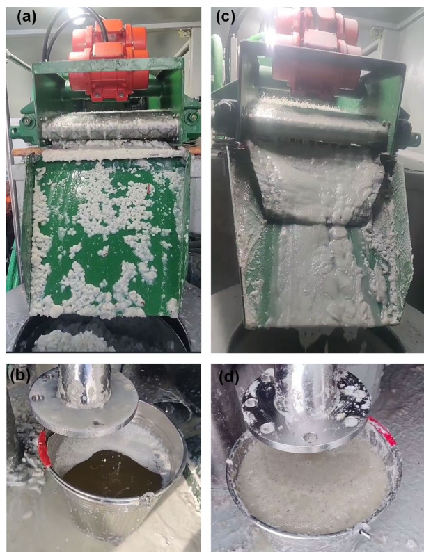
Figure 15: Performance of vibration sieve and vertical centrifuge: (a) small ball of ice chips formed on 100 meshes screen; (b) cleaned drilling fluid when using 100 meshes screen; (c) clogging of 120 meshes screen by ice chips and clay additives; (d) ice chips remaining in the drilling liquid when using 120 meshes screen.
