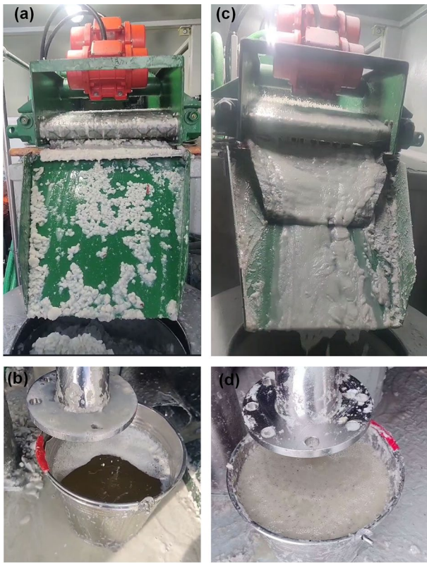
435 Figure 11: Performance of vibration sieve and vertical centrifuge: (a) small ball of ice chips formed on 100 meshes screen; (b) cleaned drilling fluid when using 100 meshes screen; (c) clogging of 120 meshes screen by ice chips and clay additives; (d) ice chips remaining in the drilling liquid when using 120 meshes screen.
