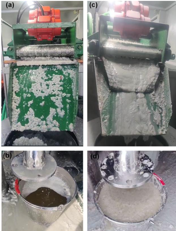
Figure 1511: Performance of vibration sieve and vertical centrifuge: (a) small ball of ice chips formed on 100 meshes screen; (b) cleaned drilling fluid when using 100 meshes screen; (c) clogging of 120 meshes screen by ice chips and clay additives; (d) ice chips remaining in the drilling liquid when using 120 meshes screen.
