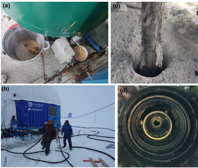
510 Figure 9: Test phenomena: (a) cyclone dust collector worked well in domestic test; (b) condensed water could not be discharged from the receiver; (c) burying the rubber hose into snow to cool compressed air; (d) condensed water refrozen on the outer surface drill pipe; (e) ice plug formed in drill pipe.
