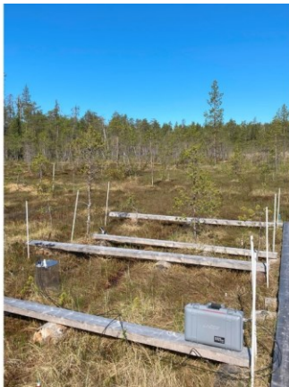
Figure 2. A flux measurement carried out with (a) a portable LI-COR Trace Gas Analyzer and (b) a clear plexiglas polycarbonate chamber placed on a round collar installed at each plot in 2020. Photos by Eeva Järvi-Laturi.
