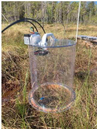
Figure 2. A flux measurement carried out with (a) a portable LI-COR Trace Gas Analyzer and (b) a clear plexiglas polycarbonate chamber placed on a round collar installed at each plot in 2020. Photos by Eeva Järvi-Laturi.
