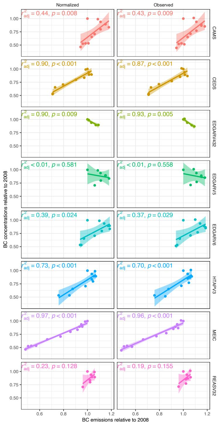
**Figure S8** Scatterplot between observed and weather normalized BC concentrations and their emissions from different inventories.
