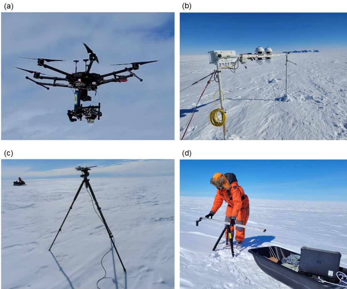
Figure 5: a) Hyperspectral camera and CM11 pyranometer in a drone, b) Eppley radiation station, c) removable 205 CM14 station, and d) ASD spectrometer.
