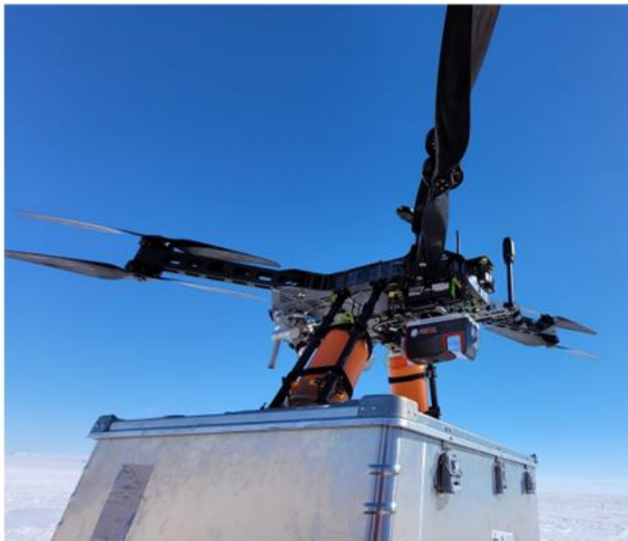
Figure 3: a) Avartek Boxer and b) Riegl VUX-120 laser scanner mounted on the front of Avartek Boxer drone, GNSS-IMU unit is located right behind the scanner, antenna is seen at the front of the scanner.
