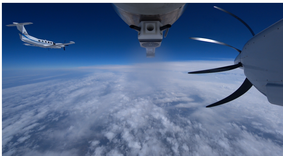
Figure 1. A picture taken from the Egrett's left landing gear camera, with the propeller of the Egrett (on the right) and the CAPS probe (on the top), shortly before going into formation flight with the Cheyenne Piper (Cheyenne 400LS registered 30 N92EV). The emission aircraft equipped with a two-engine turboprop of type Garrett/Honeywell TPE 331-14 was chased at altitudes between 7.6 and 10.4 km.
