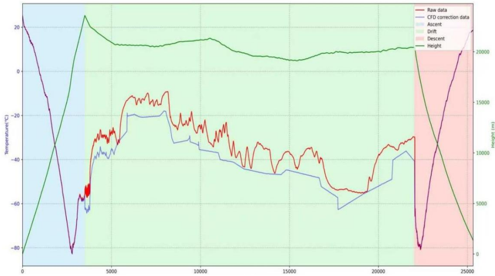
Fig. R5 decreased effect of radiation error during one observation process of ADDRS.
