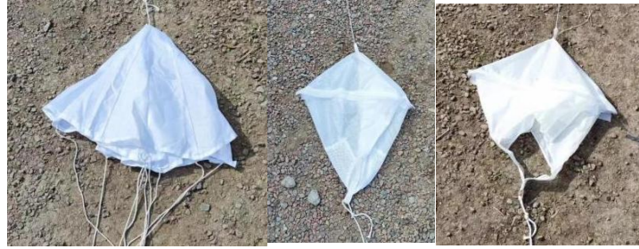
Fig.R6 Physical images of conventional parachute, small conical parachute, large conical parachute.
